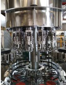
Bertolaso. We visited a manufacturer of industrial filling and processing of glass bottles. In their production line we could see advanced technology: assembly with a large scale of different mechanical parts and the automation with various industrial bus systems. Industrial ethernet, ASI-bus and Profi-Net were integrated in one control system.
